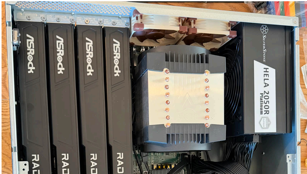
The build: the real thing, with its four cards, cooler, rear fans and power supply.
